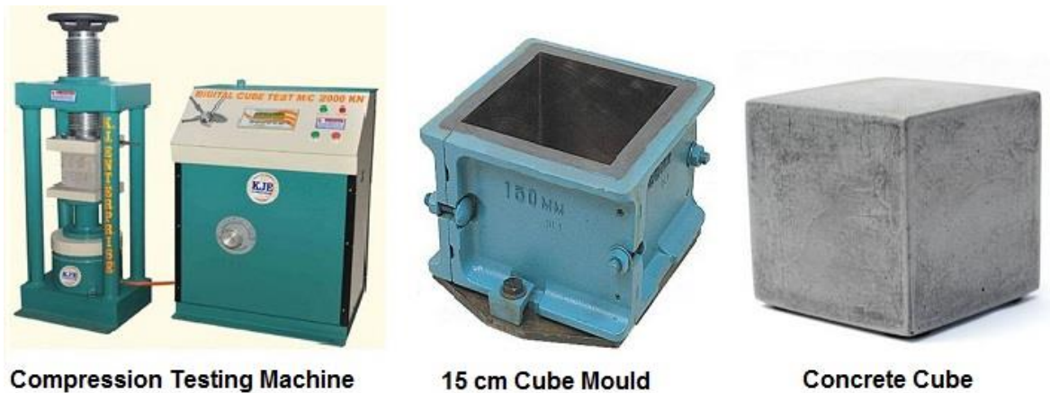
Figure 0.3: Compressive strength test
