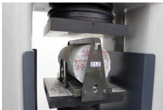
Figure 0.4: Split tensile test
